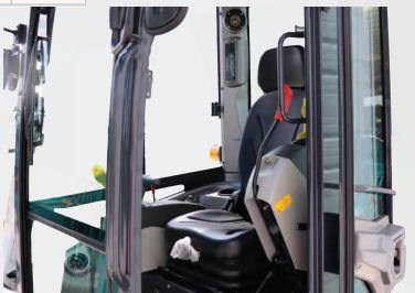
Enlcosed cab offers removable windshield and sliding windows for airflow
