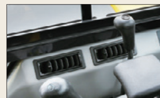
Heater with fresh air vents
