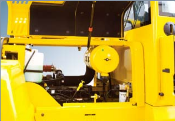
Large Engine Hood Highly accessible engine compartment assures fast and efficient maintenance.
