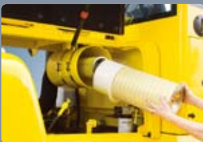
Easy Change Air Cleaner This air filter is readily accessible for cleaning or replacement.
