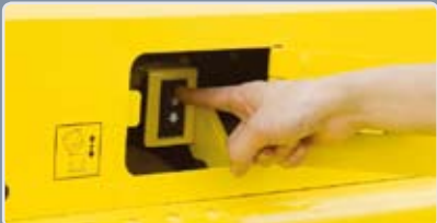
Cabin Tilting Automatic System Cabin tilting automatic system makes servicing of all power train components quick and easy. An electrically assisted hydraulic actuated cylinder tilts operator cabin to left side about 65 degrees for easy access to inside of truck components.
